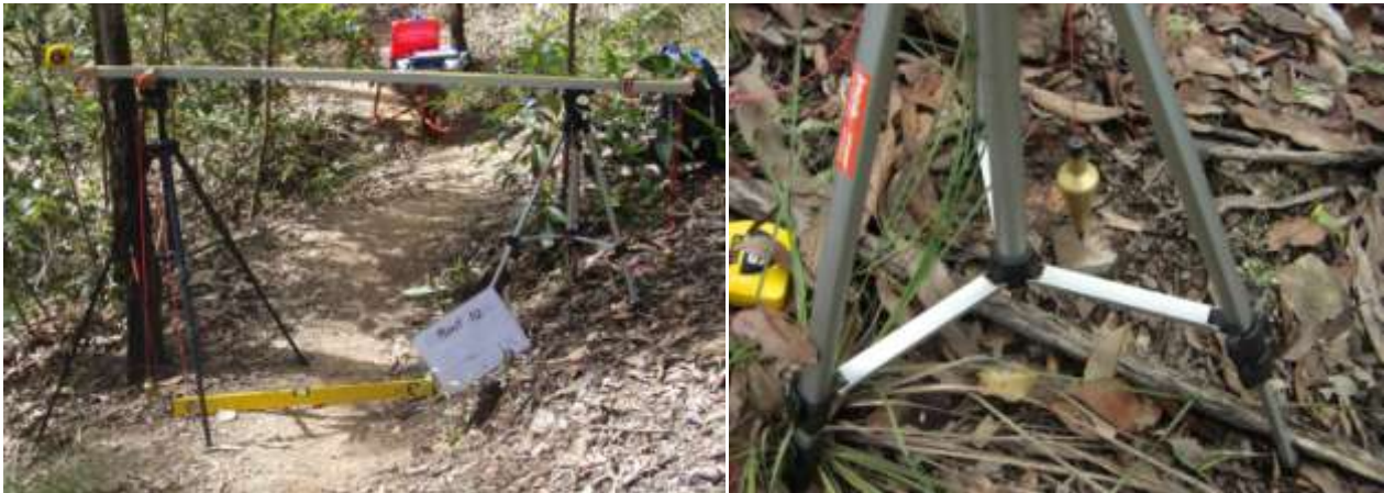
Figure 1 Transect profile measurement setup
